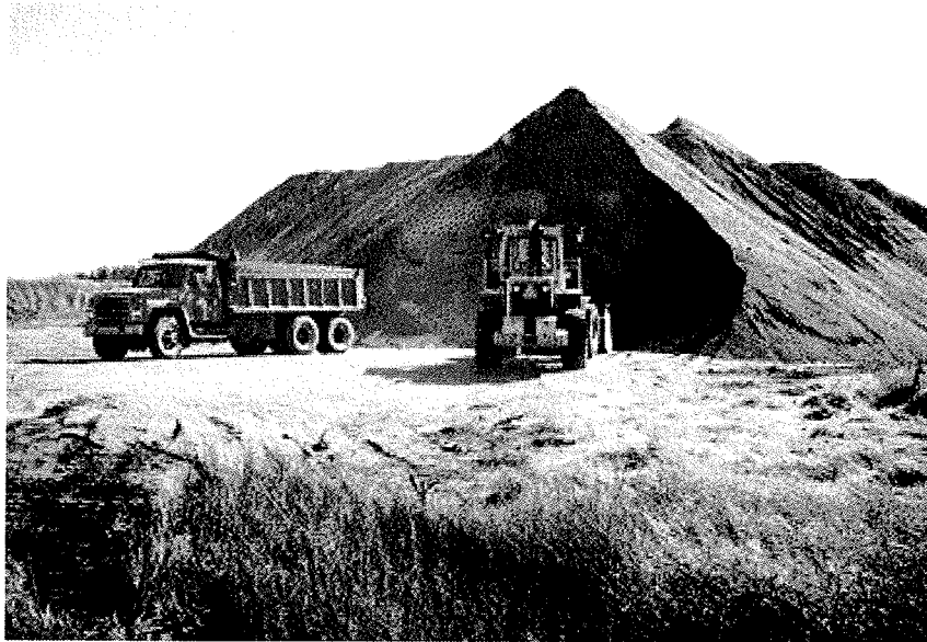
A good example of loader operation — working uniformly across the end of the stockpile. Note also a very level stockpile site and a well maintained loading area on which the loader and trucks work. This demonstrates pride in doing a good job of handling material.
