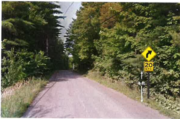
Figure 8: Curve Ahead supplemented with a 20-mph advisory speed limit plaque
