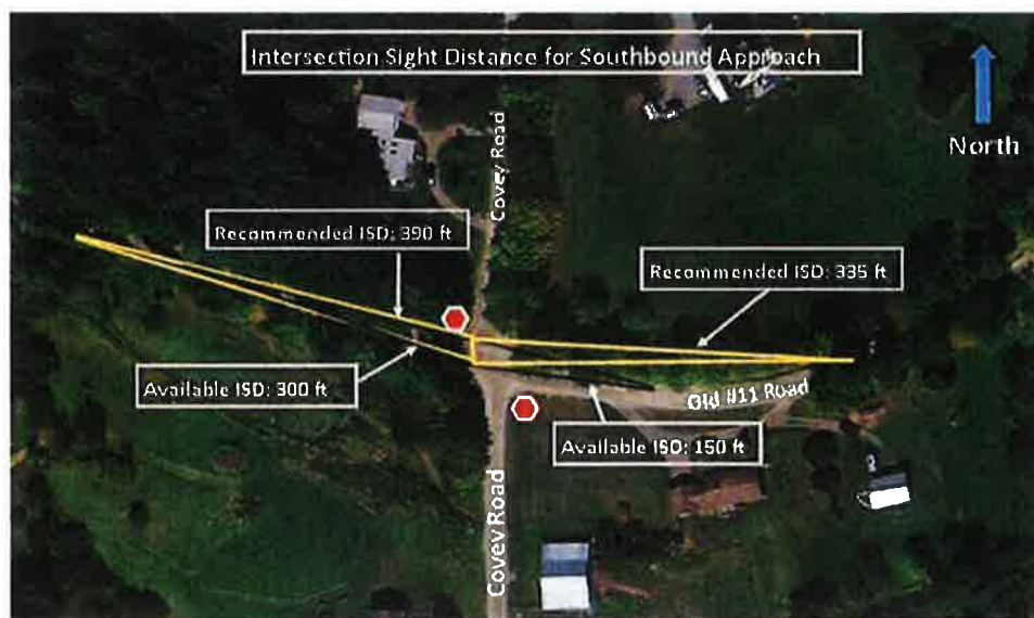
Figure 3: Intersection Sight Distance Triangle for Southbound Approach
