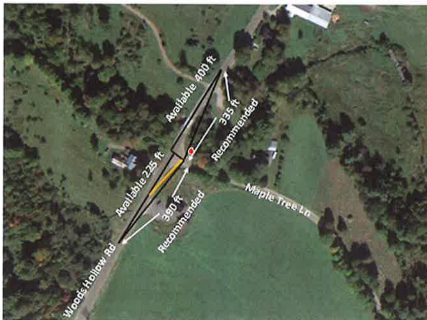
Figure 7: Sight Triangle legs at Maple Tree Ln and Woods Hollow Road
