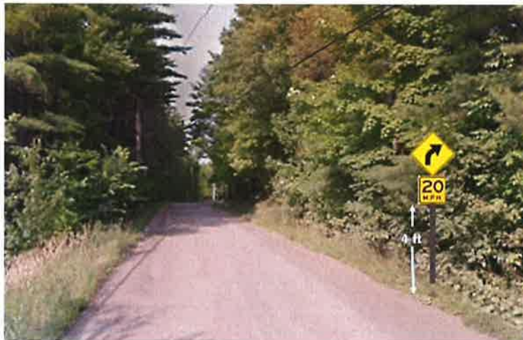
Figure 8: Curve Ahead supplemented with a 20-mph advisory speed limit plaque
