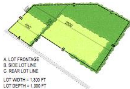
Figure 5-1. Lot Lines and Measurements
